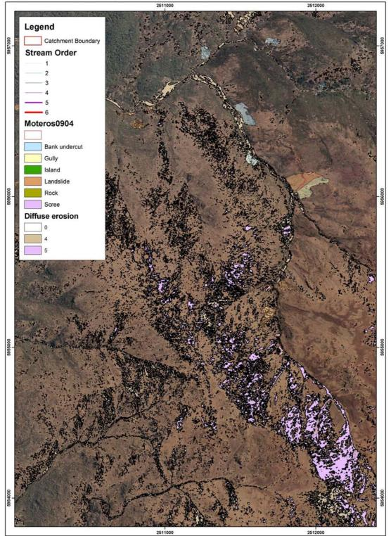
Fig. 10 Mapping of erosion features in the headwaters of the Motueka River (this map shows the delineation of diffuse erosion and point sources such as gullies and landslides)
