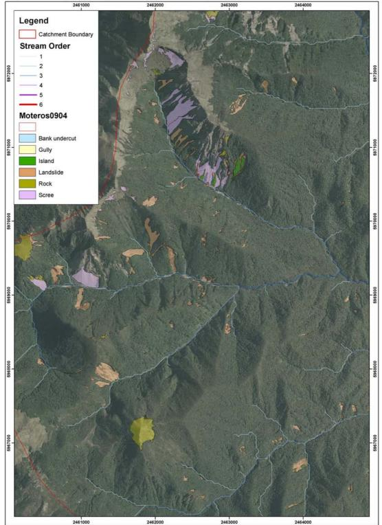
Fig. 9 Mapping of erosion features in a forested area of the headwaters of the Wangapeka
