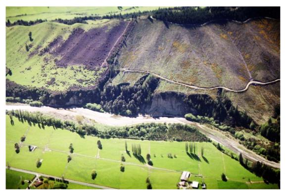
Fig. 7 Severe bank erosion in the Motupiko River near Quinneys Bush
