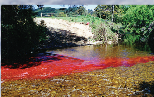
Dye test, Sherry River. The non-toxic dye rhodamine WT was used to measure travel time (2.21 min) from ford to monitoring site (60 m downstream) and to ensure full mixing at the monitoring point.
