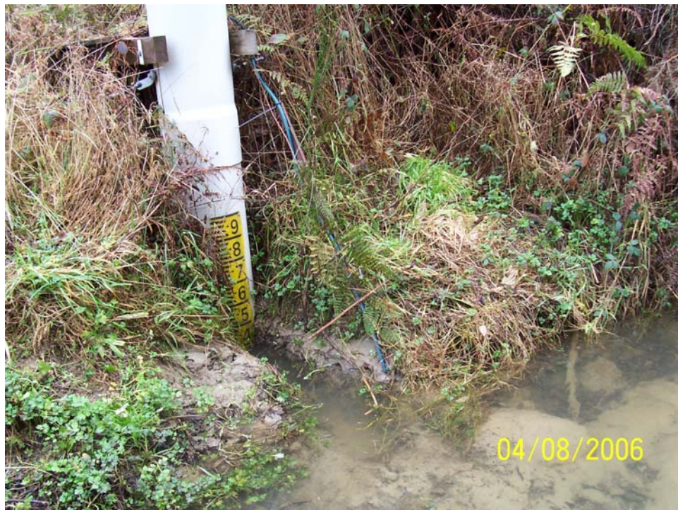
Figure 1.3a and b: Herring at Recorder. The auto-sampler is located on the catwalk of the logger housing (the tower and housing were painted green 2007). The auto-sampler hosing and turbidity sensor are strapped to waratah slightly upstream of the static tube. It can be seen from the lower photo that the hose, sensor and static tube were prone to silting up.
