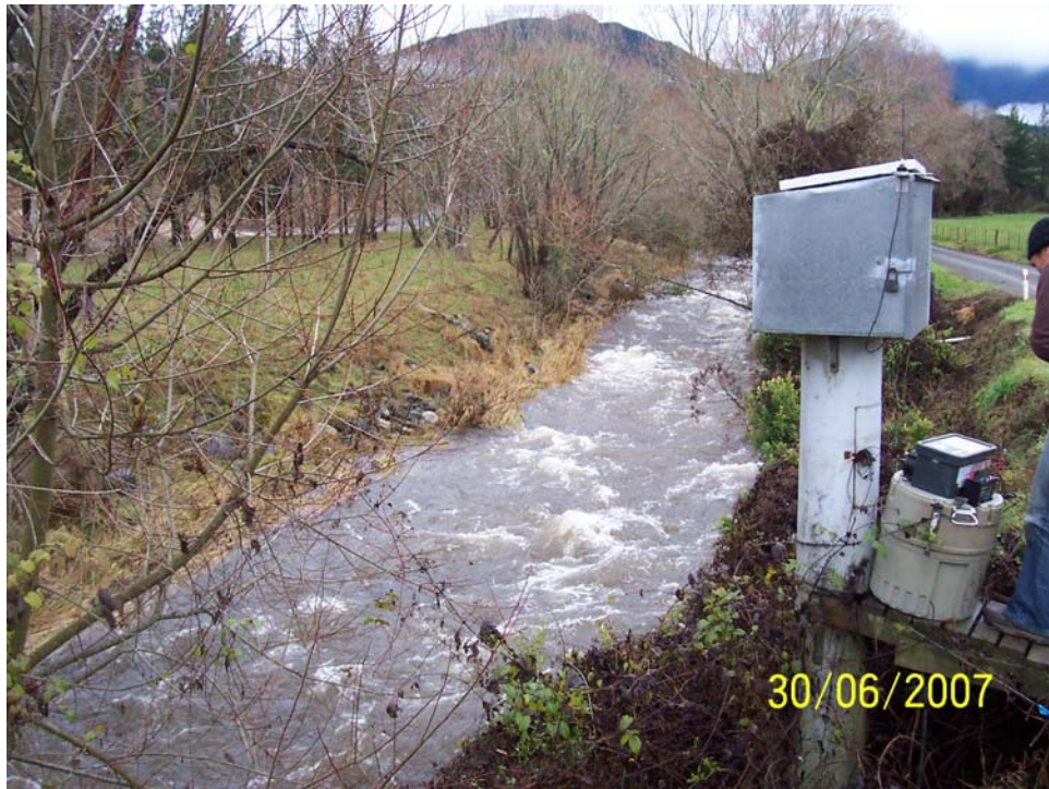
Figure 1.2: Big Pokororo at Recorder. The auto-sampler hose and turbidity are tied off to a waratah 1.5 meters upstream of the water level static tube.
