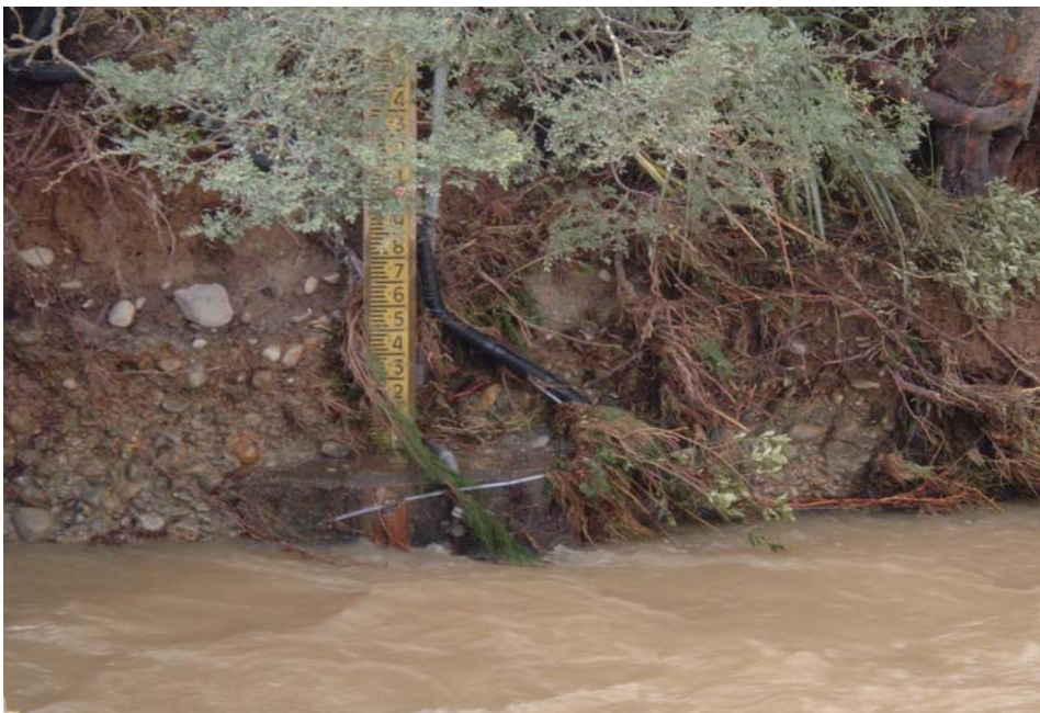
Figure 1.1: Motupiko at Christie's original site. On top photograph, turbidity sensor is to left of staff gauge, auto-sampler intake pipe is to right. Bottom photograph shows the site after the Easter 2005 flood washed away the monitoring equipment.
