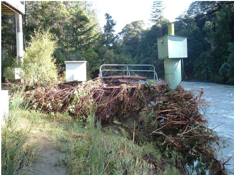
Figure 1.5b: Motueka at Gorge. Grey box holds battery and data-logger. Top photograph shows the auto-sampler under the walkway. Bottom photograph shows debris from Easter 2005 flooding.
