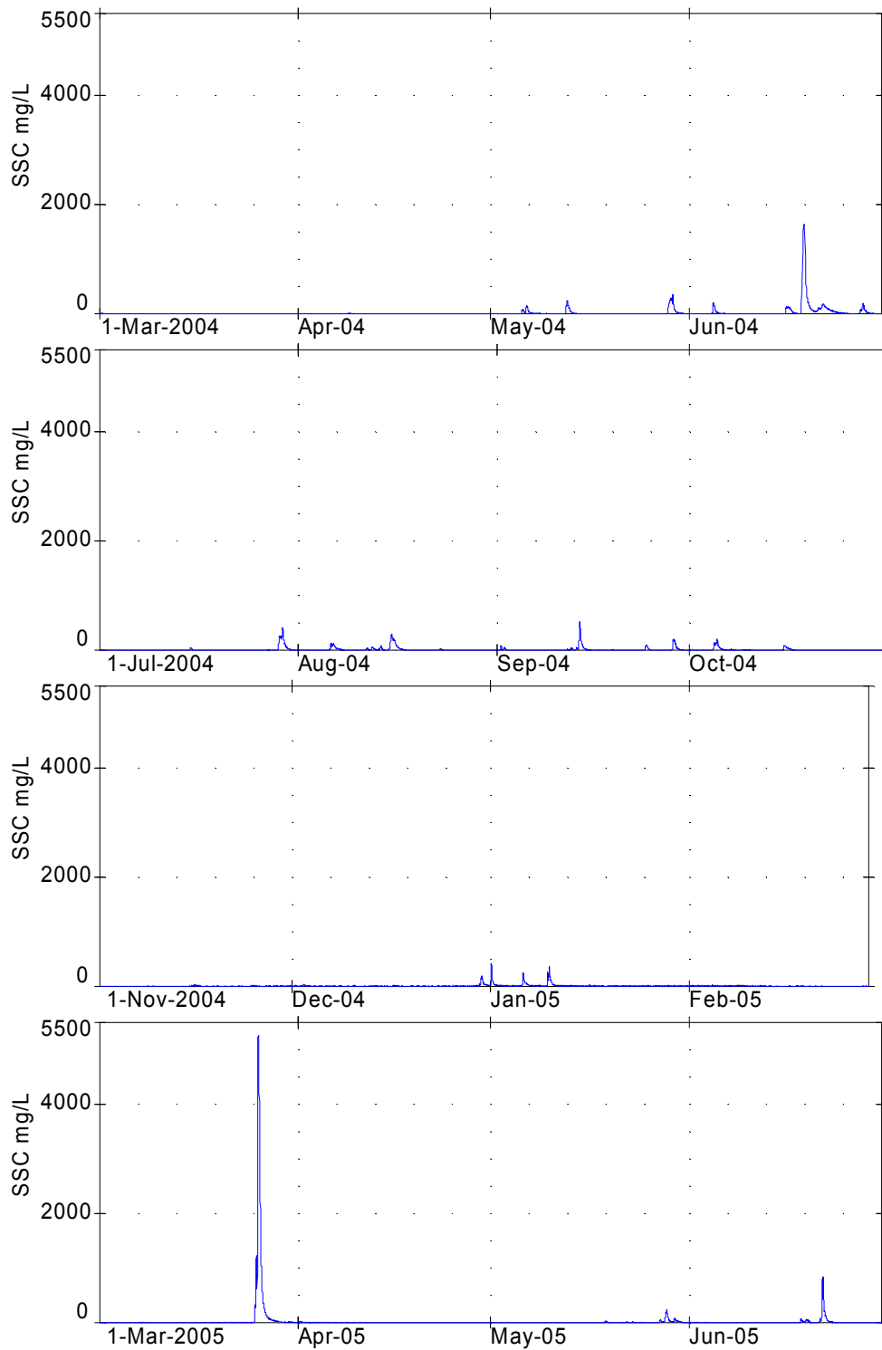
Figure A8.2: Derived suspended sediment concentration (SSC, mg/L) record, 1 March 2004 to 1 July 2005 at Motueka at Woodman's Bend.
