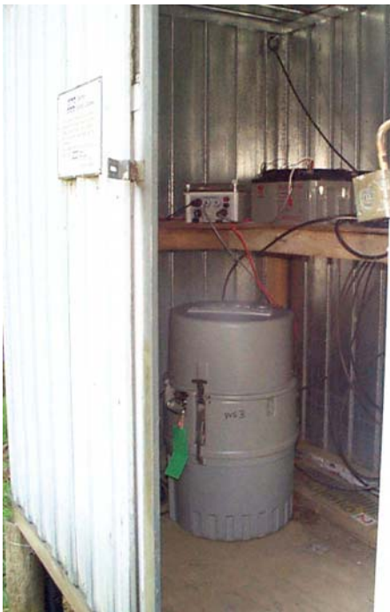
Figure 1.3: Wangapeka at Walter Peak. The turbidity sensor and stage sensor are in the white plastic tube. The auto-sampler intake hose runs through the steel pipe several metres downstream.
