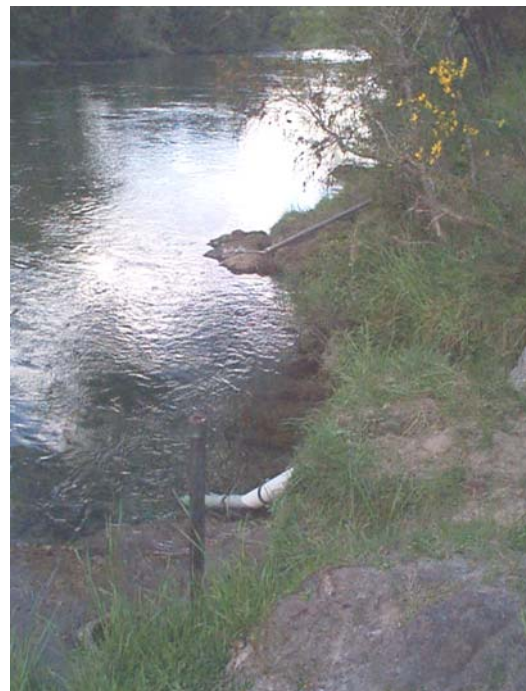
Figure 1.3: Wangapeka at Walter Peak. The turbidity sensor and stage sensor are in the white plastic tube. The auto-sampler intake hose runs through the steel pipe several metres downstream.
