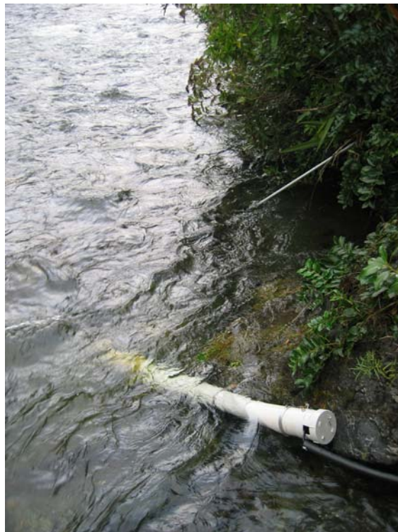
Figure 1.5a: Motueka at Gorge. Turbidity sensor is hidden within plastic tube, while steel pipe is linked to auto-sampler.
