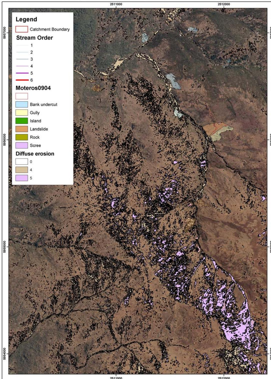
Fig. 10 Mapping of erosion features in the headwaters of the Motueka River (this map shows the delineation of diffuse erosion and point sources such as gullies and landslides)
