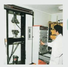
Root tensile strength testing was carried out using a Floor Model 1195 Instron Universal Testing Machine
